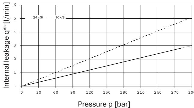
Do not operate pump more than 5 seconds at any speed or viscosity if internal leakage is higher than 50% of theoretical flow.
