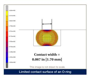
Taking into consideration materials used as well as the geometries of the mating surfaces, TechSeal's team of Application Engineers can perform an FEA simmulation to test the PiP seal's behavior under various conditions, ensuring a good fit across all tolerance ranges. For more information please contact TechSeal's Application Engineering team.
