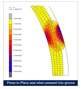
As a precision cut seal, the PiP seal still maintains its rectangular cross section, providing a maximum sealing surface. A wider contact surface can compensate for more imperfections in stamped or cast mating components. The two FEA simulations below demonstrate the wider contact area of a precision cut PiP than that of an O-ring.
