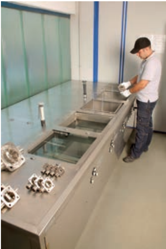
Ultrasonic cleaning of valve bodies
