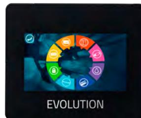
Thanks to SITA PLC, TOUCH SCREEN and new generation lamp drivers you can regulate lamp power manually or automatically to reach required disinfection rate. All PR UNITS can be connected to flow meter and UV transmittance sensor.
